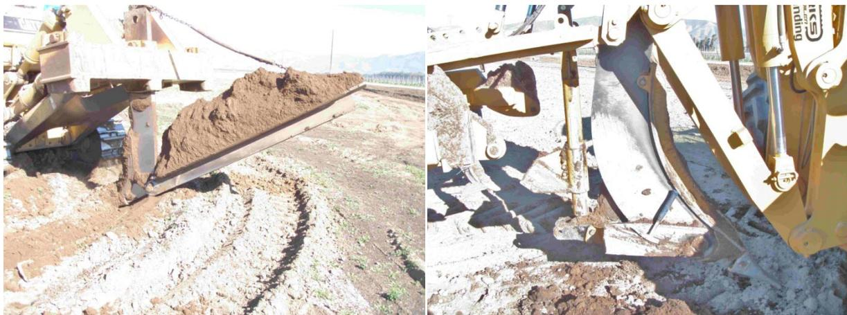
Figure: 1 Standard slip plow (left) and a SoilWorks “Curved Flat 700 mm” Vibrosoiler with low-set secondary wing (right).
